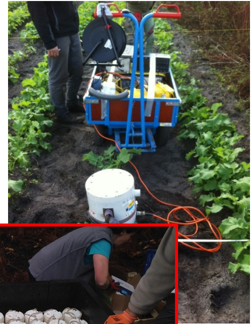
(b) Line array with GFZ geophones (c) Vibrometer source ( > 15 Hz)
