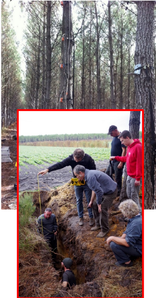
Tree instrumented with 6 velocimeters
